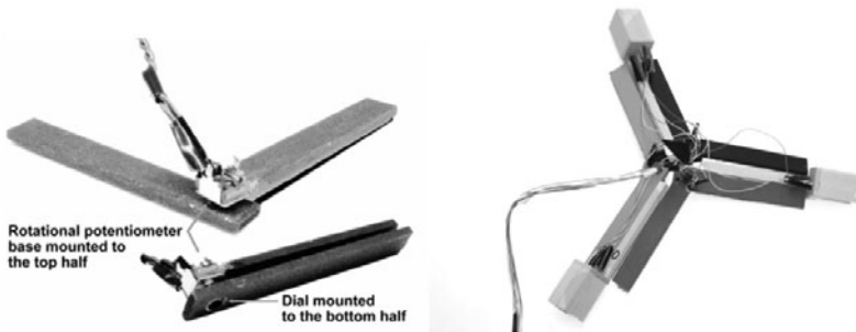
◀ Figure 16: (left) Rotational potentiometer mounted to a hinge. (right) Flexible hub with rotational potentiometers.
