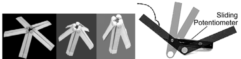
► Figure 14: (left) Flexible hinge concept. (right) Sliding potentiometer measuring the angle bend.
