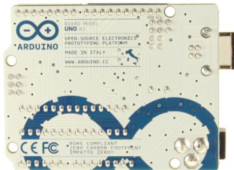
**Be aware that the back side of the board has no insulation, Do not place it directly on the metal table. (It may not work Properly or even destroy the Arduino)**
